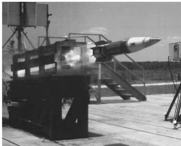
Fig. 22 Flight test of CKEM laser window configuration.
